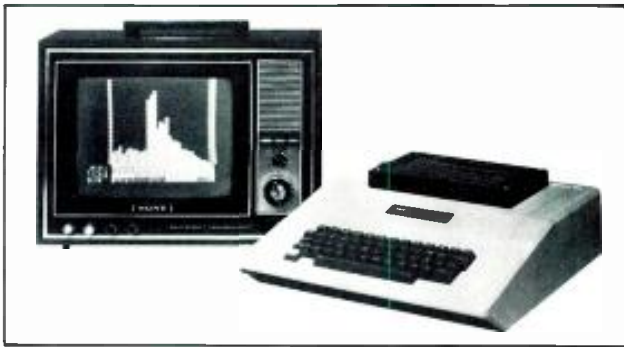
Eventide's APX252 Real Time Spectrum Analyzer.
